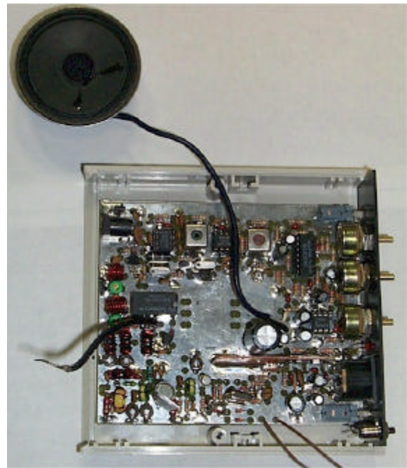
Fig 2: Partial Assembly Testing Receiver Section
