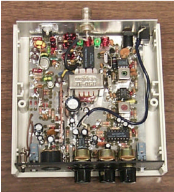
Fig 1: 6M AM Transceiver With Cover Removed
