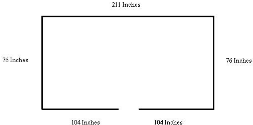
Figure 1. The original loop designed for 15 meter operation.
